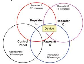
• In example 2, the sensor could be added to wireless repeater A, B, or C. Since repeater A and B are closer to the alarm panel, the sensor should be added to either repeater A or B.
